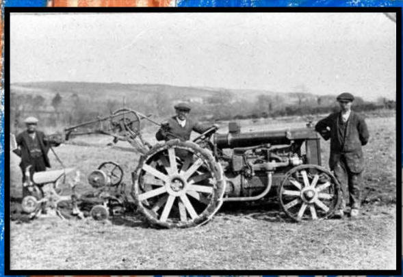
Above: whilst photographed in Kings Nympton, our archive tells us that this tractor was manufactured in South Molton as follows: 'Fordson tractor with one of the first tractor ploughs, made by Bawden's of South Molton. Produced from 1917. The British government, anxious to secure supplies of tractors and implements to help the food production campaign of the First W.W, placed an order for 6,000 of these tractors. It was a successful choice, for the Fordson was on the whole reliable, sturdy and efficient.' Date unknown.
